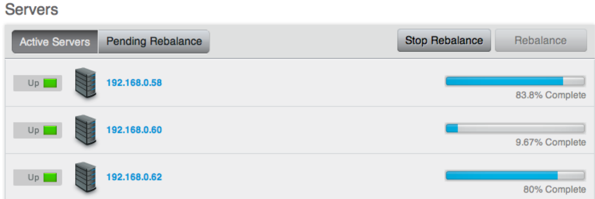
Figure 2.11. Online Upgrade — Starting the Rebalance Process
